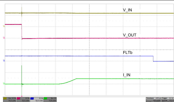
Figure 7-27. Hot-Short: Fast Trip Response and Current Regulation
