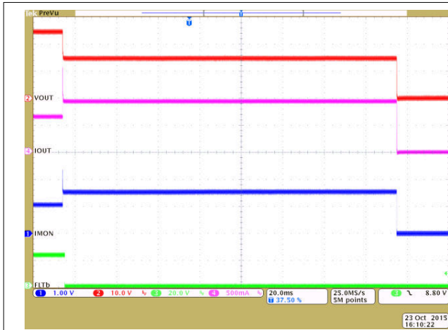
RILIM = 12 k \Omega RILIM = 12 k \Omega Load transient event MODE pin connected MODE pin connected to RTN to RTN
