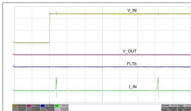
Figure 10-13. Turnon With Short Circuit on Output
