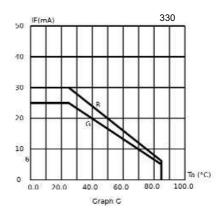
^ = Products must be derated according to the derating information. Each derating graph refers to specific LEDs.
