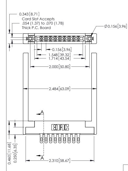
SECTION A-A 0.295 [7.49] Card Slot 0.165[4.19] Point of Contact
