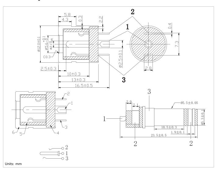
**tolerance** X: ±0.5 mm .X: ±0.3 mm .XX: ±0.05 mm applicable unless otherwise indicated in specification or on drawings
