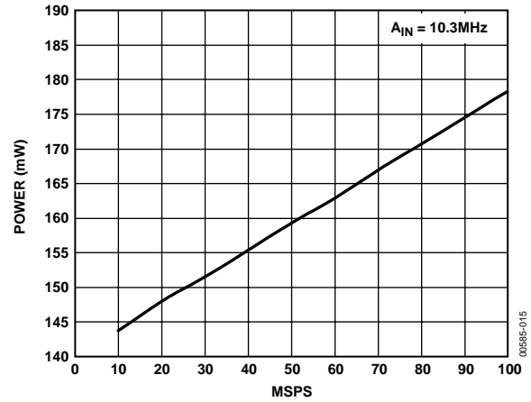
Figure 15. Analog Power Dissipation vs. Encode Rate
