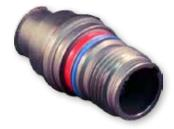
Series 881 threaded coupling cable receptacle with solder cup contacts for soldering to wires. Thread-on rear adapter allows access to contacts. Install cable shield braid directly to connector with Band-Master Micro band. Three contact sizes are available with current ratings of 5A, 3A and 1A. Aluminum or stainless steel housings and thermoplastic insulators. Ultraminiature SuperFly® connectors are ideal for soldier systems and other applications where reduced size and weight are a must.
