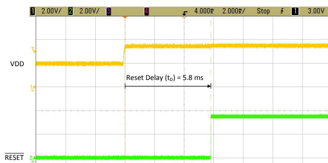
Figure 54. TPS3840EVM \overline{\text{RESET}} Time Delay ( t_D ) with 0.01- \mu\text{F} Capacitor
