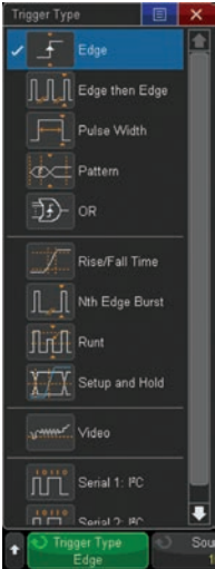
Figure 43. Wide array of advanced parametric trigger modes.
