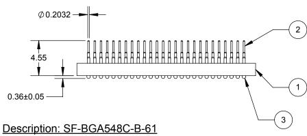
Primary dimension units are millimeters, Secondary dimension units are [inches], Weight is in grams. Tolerances: Hole diameters ±0.0254mm [±0.001"], Pitches (from true position) ±0.0254mm [±0.001"], substrate thickness tolerance ±10%, all other tolerances ±0.127mm [±0.005"] unless stated otherwise. Materials and specifications are subject to change without notice.
