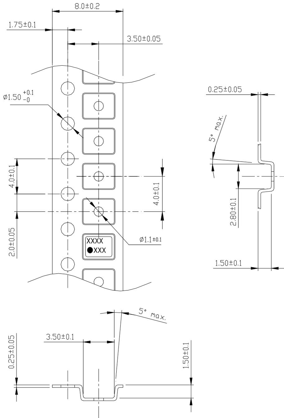
1. Clearance of an embossing tape, and a product unit: mm
