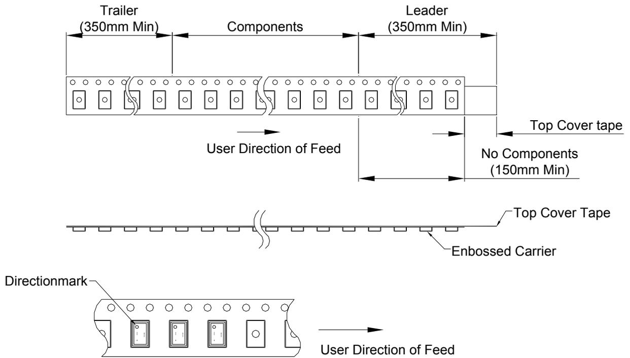
When a tape end is taken out to the front, sprocket holes becomes right hand side.
