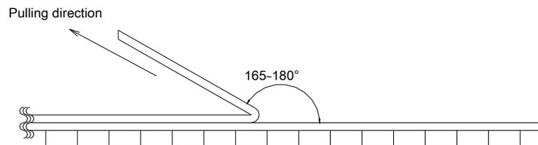
Fig.2. Taping specification
