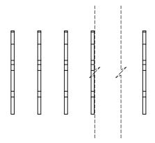
NOTE: CONTACTS ARE HELD IN A CARRIER FOR EASE OF ASSEMBLY
