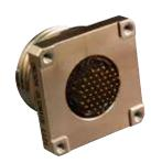
Rear Panel mount jam nut receptacle features square flange for secure attachement of rigid boards or flex circuits. Flange has #2-56 stainless steel helicoils and integral standoffs. PC tail contacts are facotry installed, potte with epoxy and are nonremovable. Gold–plated copper alloy contacts, aluminum or stainless steel shell, fluorosilicone seals and LCP insulators
