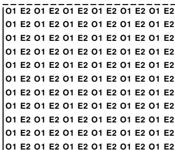
Figure 15. Combine Frame Output from Graphics Controller
