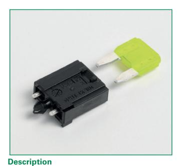
Fuse holder for MINI/ FK1 fuses for PCB applications. The FL1 Fuse Holder can be mounted in a row of nearly any number. The terminals fit into a 7.62 mm pitch.
