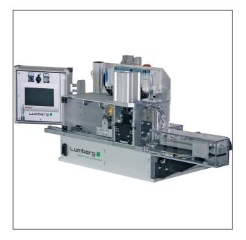
Semiautomatic harnessing machine for termination of RAST 2.5 connectors in insulation displacement technology, larger base machine, with integrated stations for cable color detection and keying cutting, individual upgrading possible
