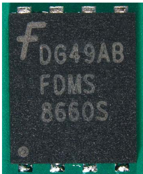
Figure 1: Power56 Mounted on PWB
