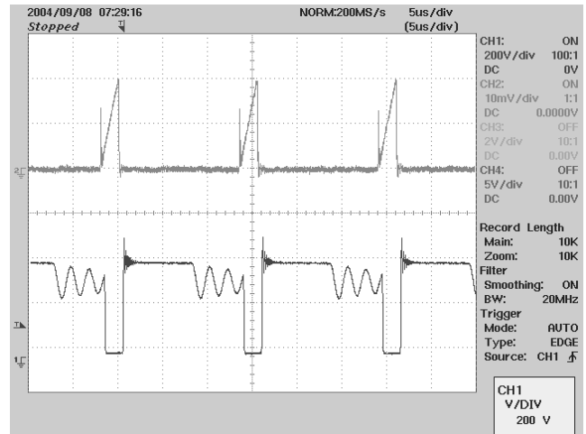
Figure 11 - 265 VAC, Full Load Upper: I_{DRAIN} , 0.5 A / div Lower: V_{DRAIN} , 200 V / div, 5 \mu s / div
