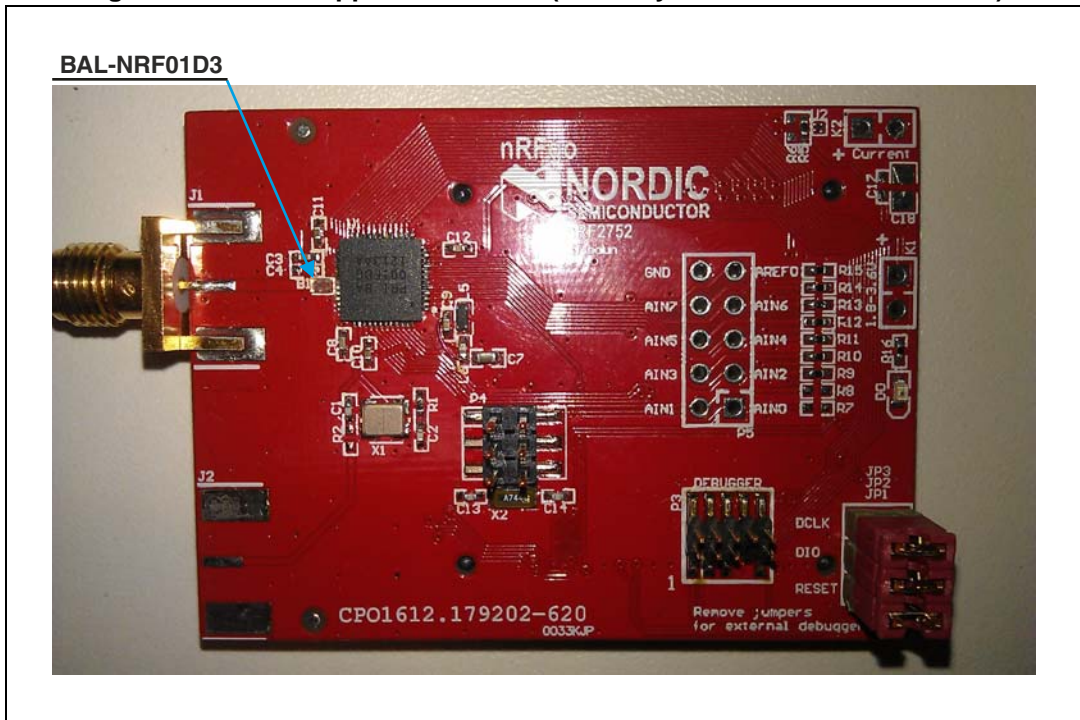
Figure 9. nRF2752 application board (courtesy of Nordic Semiconductor)
