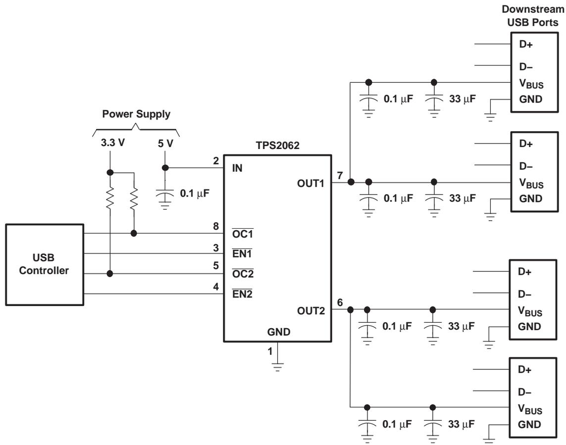
Figure 27. Typical Four-Port USB Host / Self-Powered Hub
