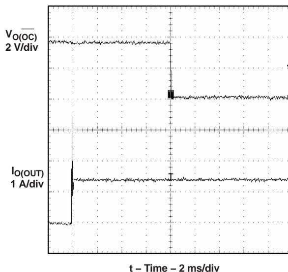
Figure 9. 1-Ω Load Connected to Enabled Device
