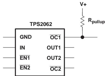
Figure 26. Typical Circuit for the  $\overline{OC}$  Pin
