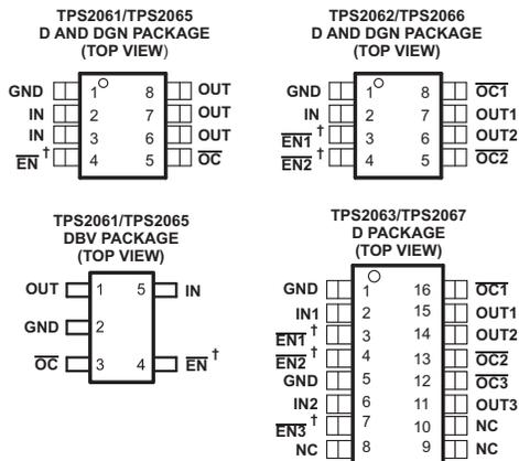
† All Enable Inputs Are Active High For TPS2065, TPS2066, and TPS2067
