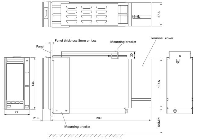
Note) The distance between other instruments and low end of PDJ shall be more than 100mm.
