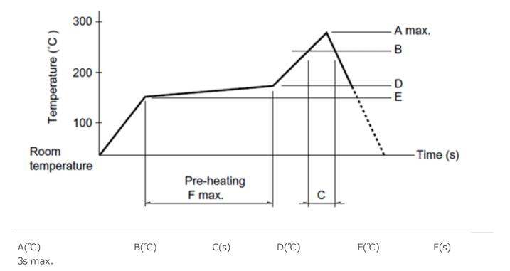
(1) The condition mentioned above is the temperature on the mounting surface of a PC board. There are cases where the PC board's temperature greatly differs from that of the switch, surface depending on the PC board's material, size, thickness, etc. The above-stated conditions shall also apply to switch surface temperatures.
