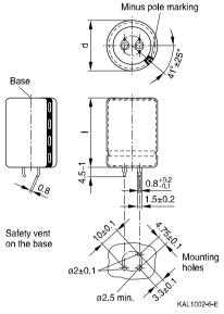
Snap-in capacitors are also available with 3 terminals (length 4.5-1 mm). For packing mode and ordering example see next page.
