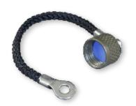
Protective covers fit Series 800 plug and receptacle connectors. Aluminum or stainless steel. Fluorosilicone rubber gasket protects connector from contamination and water ingress. Attach to panel or cable with a variety of lanyards and fittings. Lanyard styles include braided nylon rope, stainless steel wire or sash chain. Stainless steel wire available with flexible, rugged polyurethane coating or Teflon™ sleeve for high temperature requirements.
