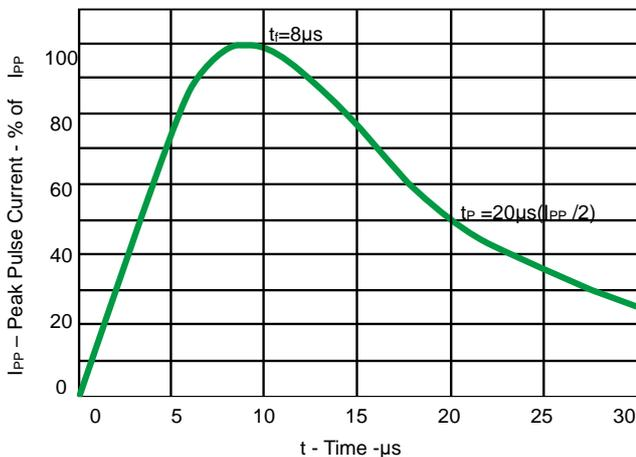
Fig 1.Pulse Waveform
