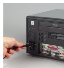
Plug ring-lock securely fastens the power cord
