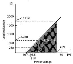
Note: For communication with FXW, min. of 250  $\Omega$  required.
