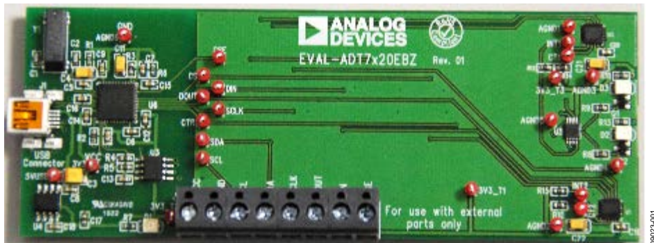
Figure 1. ADT7x20 Evaluation Board—Main Board
