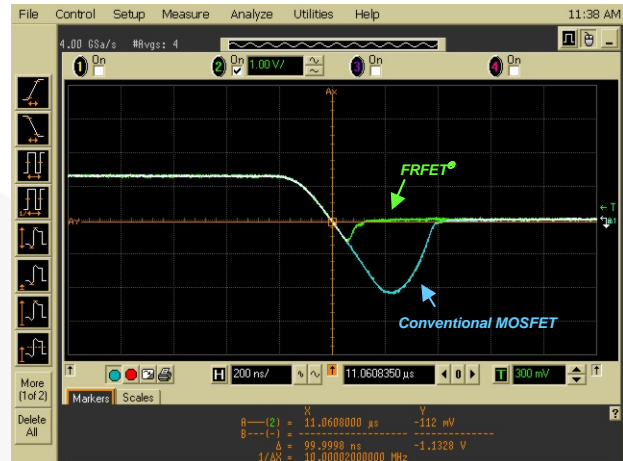
Figure 23. Comparisons of Reverse Recovery Characteristics Between FRFET® and Conventional MOSFET
