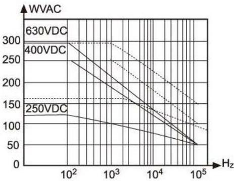
Working Voltage DC&AC vs. Frequency
