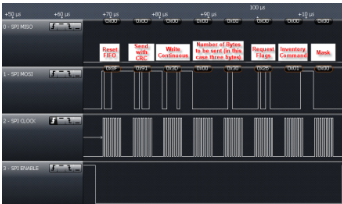
Figure 6-22. Inventory Command Sent From MCU to TRF7970A
