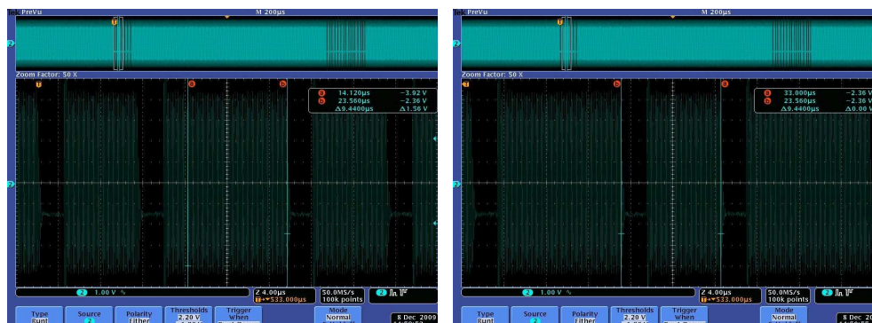
Figure 6-31. Receive Data Bits and Framing Level
