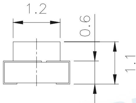
For Reflow Soldering (propose)
