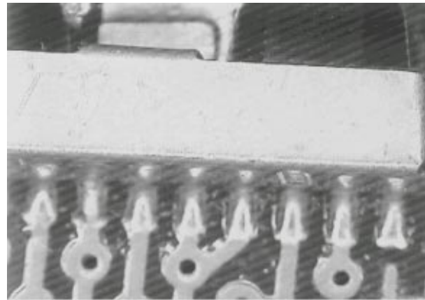
Photo 4.0. Unit self-aligns after reflow.
