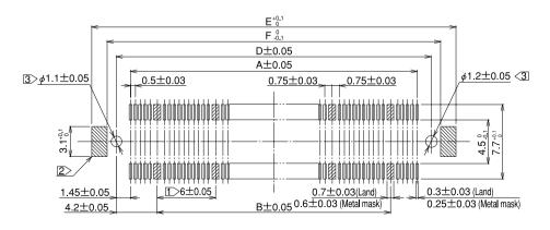
Note 1 Cross-hatched portions, totaling n places, indicate the ground circuits.
