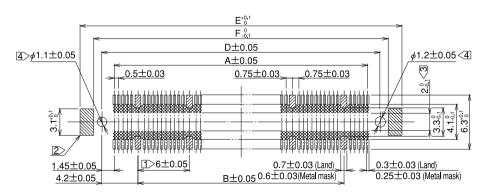
Note 1 Cross-hatched portions, totaling n places, indicate the ground circuits.
