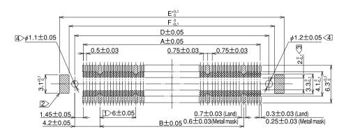
Note 1 Cross-hatched portions, totaling n places, indicate the ground circuits.
