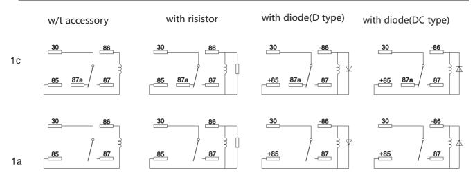
Wiring Diagram (bottom view)
