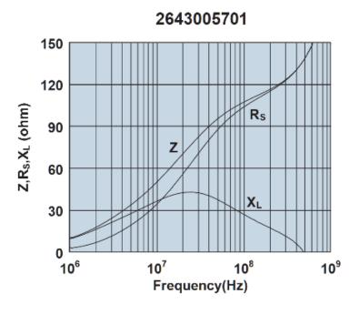
Impedance, reactance, and resistance vs. frequency.
