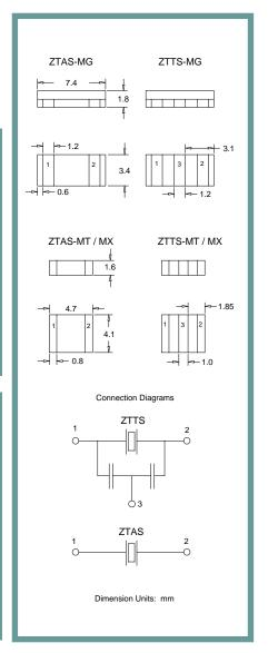
The terminations of the ZTAS and ZTTS series ceramic resonator are Pb free. Pb may be contained in the ceramic resonator element of this device and is exempted via item 7 of the RoHS annex. This ceramic resonator series is considered RoHS compliant.
