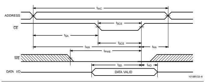
Write Cycle No. 2 (WE Controlled, OE HIGH During Write)[12, 13]
