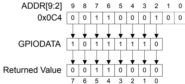
Figure 8-3. GPIO DATA Read Example
