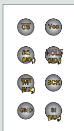
Figure 1-3. 8-ball WLCSP (Bottom View)
