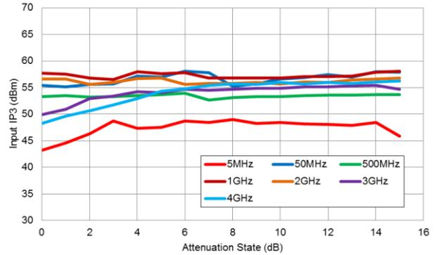
**Input IP3 versus Attenuation State**
