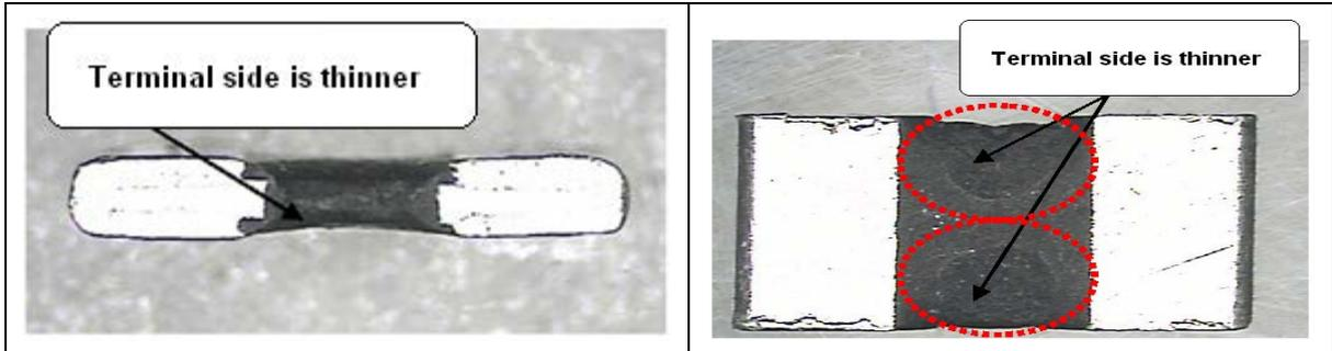
10.3.2 When customer performs wave solder process shall take note on the dispensing gap.
