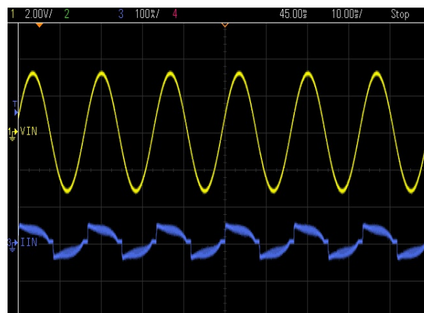
Figure 12. Input AC voltage vs. input AC current
