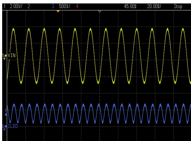
Figure 11. Input AC voltage vs. output current
