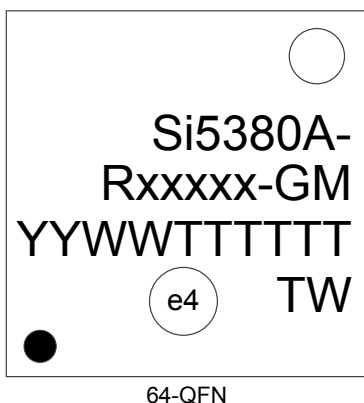
Figure 12.1. Si5380 Top Marking
