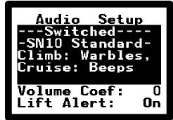
In climb, the SN10 standard audio makes a nice warble sound increasing both pitch and warble rate with climb. It becomes a sad solid tone decreasing in pitch as climb drops below zero. In cruise the audio gives speed-to-fly; an interrupted tone means slow up, quiet means you're flying at about the correct speed, and a solid tone means speed up.
