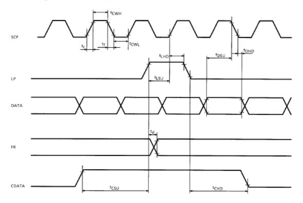
Test Conditions (Unless Otherwise Noted, V<sub>DD</sub> = 5.0 V ± 10%, V<sub>SS</sub> = 0 V, Ta = -20 to 70°C)
