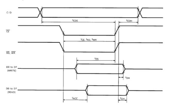
Test Conditions (Unless Otherwise Noted, V<sub>DD</sub> = 5.0 V ± 10%, V<sub>SS</sub> = 0 V, Ta = -20 to 75°C)
