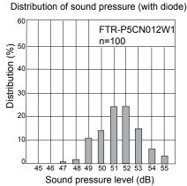
Method of acoustic noise measure Measuring condition: Distance from 5 cm, relay operation at 10Hz Tester: Noise tester Ryon NA-61, A range
