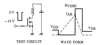
$\begin{array}{l} T_{ch} = 25^{\circ}C \ (Initial) \\ Peak \ I_{AR} = -4.5 \ A, \ R_G = 25 \ \Omega \\ V_{DD} = -24 \ V, \ L = 1.0 \ mH \end{array} \\ \begin{array}{l} E_{AS} = \frac{1}{2} \cdot L \cdot I^2 \cdot (\frac{B_{VDSS}}{B_{VDSS} - V_{DD}}) \end{array}$
