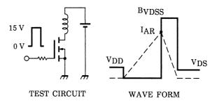
$$\begin{array}{l} T_{ch} = 25^{\circ}C \ (Initial) \\ Peak \ I_{AR} = 6 \ A, \ R_G = 25 \ \Omega \\ V_{DD} = 24 \ V, \ L = 1.0 \ mH \end{array} \\ \begin{array}{l} E_{AS} = \frac{1}{2} \cdot L \cdot I^2 \cdot ( \ \frac{BVDSS}{BVDSS} - V_{DD}) \end{array}$$
