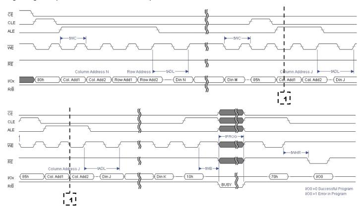
**Note:**  $t_{ADL}$  is the time from  $\overline{WE}$  rising edge of final address cycle to the  $\overline{WE}$  rising edge of first data cycle.
