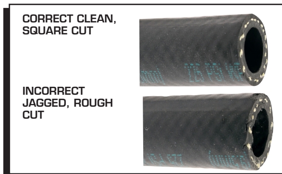
Figure 24 Severing the Hose Properly.
