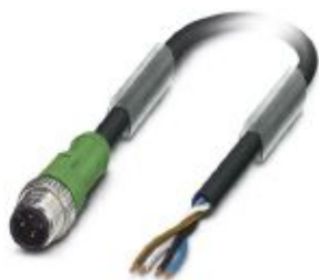
Sensor/actuator cable, 4-position, PUR, black-gray RAL 7021, Plug straight M12, coding: A, on free cable end, cable length: 10 m
